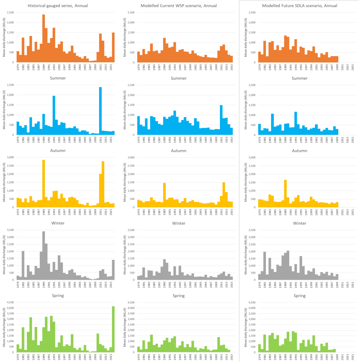
Figure 45. Historical gauged (1978 – 2016), modelled Current WSP (1978 – 2015, except spring) and modelled Future SDLA (1978 – 2009, except spring) annual and seasonal flow series for Billabong Creek @ Darlot gauge (410134).
